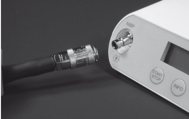
Fig. 2-3 Cuff connection of the PHYSIO-PORT devices
