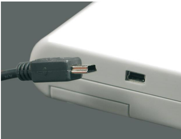
Fig. 2-4 Connection of the mini-USB connection cable
