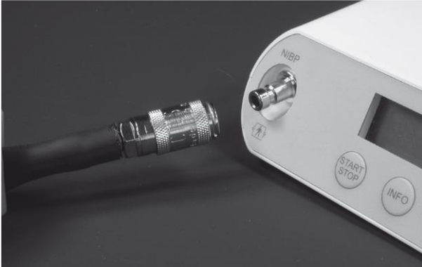
Fig. 2-3 Cuff connection of the ABPM devices
