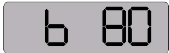
Fig. 3-6 Battery capacity of 80 %
