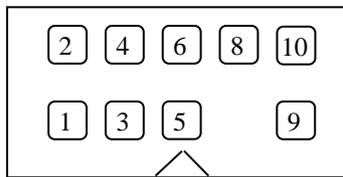
Pin 1 Power supply Pump : + 5VDC      **or**      + 12VDC
